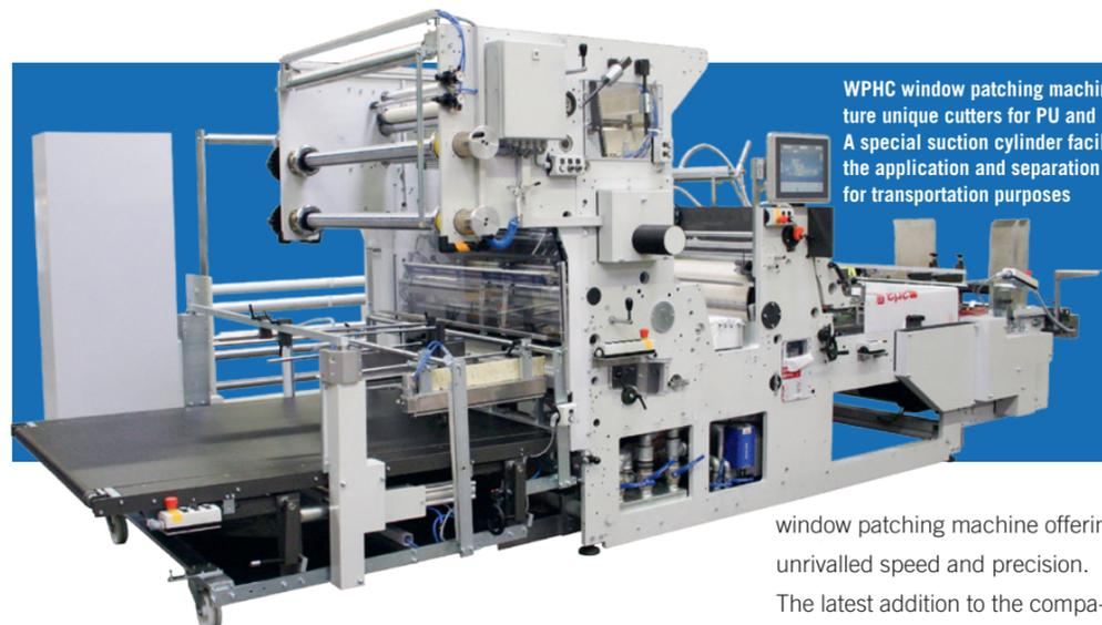
WPHC window patching machines feature unique cutters for PU and PE foils. A special suction cylinder facilitates the application and separation of foil for transportation purposes
